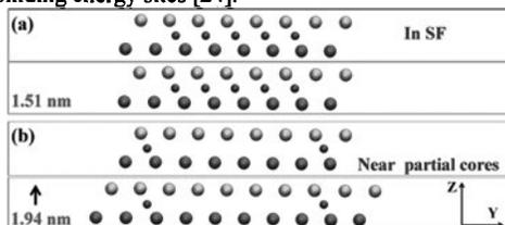
Figure 3. Initial and equilibrium configurations showing the change in the SF width of a screw: (a) H-arrays (purple spheres) in the SF; and (b) two H-arrays near the partial cores.
