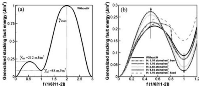
Figure 4. Generalized stacking fault energy of  $[1\bar{1}2](111)$  slip system (a) without and (b) with H.
