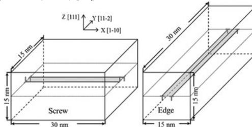
Figure 1. Schematic showing dissociated screw and edge dislocations. The Shockley partials are denoted by ‘T’ or inverse ‘T’ symbols and the shaded areas represent stacking fault.
