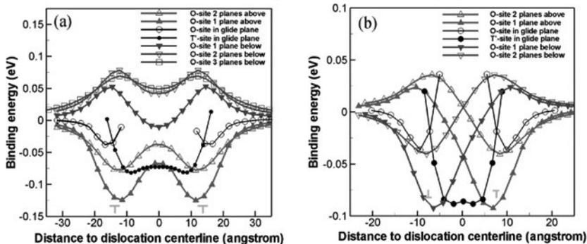
Figure 2. Binding energies of H to (a) edge; and (b) screw dislocations. The positions of the Shockley partial cores are shown by 'T' and inverse 'T' symbols.
