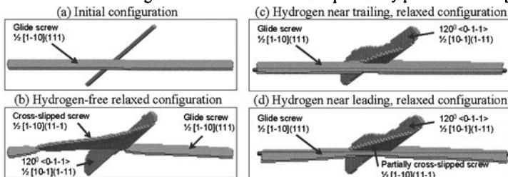
Figure 5. (a) Initial and (b) relaxed configurations showing instantaneous cross-slip; (c) and (d) relaxed configurations showing cross-slip with H-array occupying different positions.
